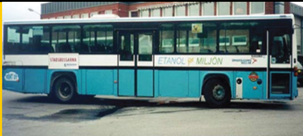
Figure 1 Ethanol city bus commuted into city area and reached 1 million kilometer during the period of year 1986-2000 or after 14 years [2]
