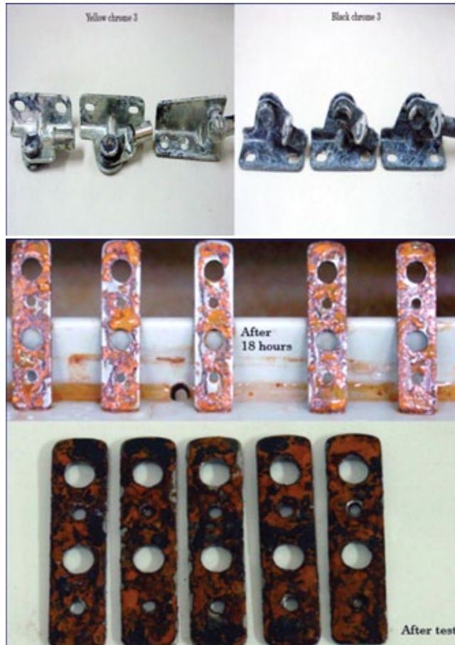
Figure 3 show the testing result of white rust and rust
