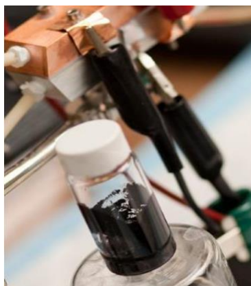
รูปที่ 2-6 'Cambridge crude' — a black, gooey substance that can power a highly efficient new type of battery. A prototype of the semi-solid flow battery is seen behind the flask." โดย Dominick Reuter [11]
